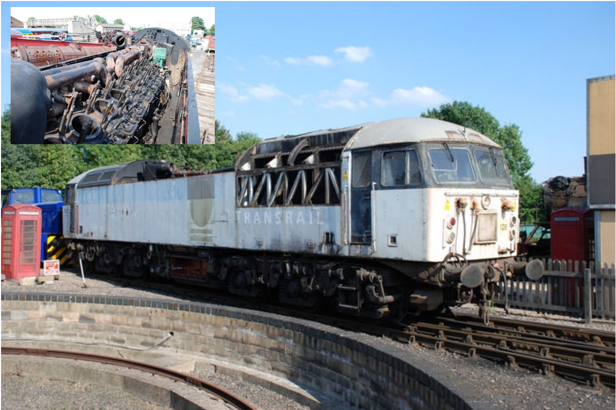
56128 at Wansford 24/07/08 with (insert) all 16 cylinder heads exposed whilst the engine receives a top end overhaul Photos: Hanson Traction Ltd
